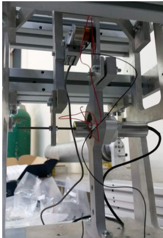
Figure 2.30. Initial calibration mechanism design with load cell and voice coil, and LVDT assembly
