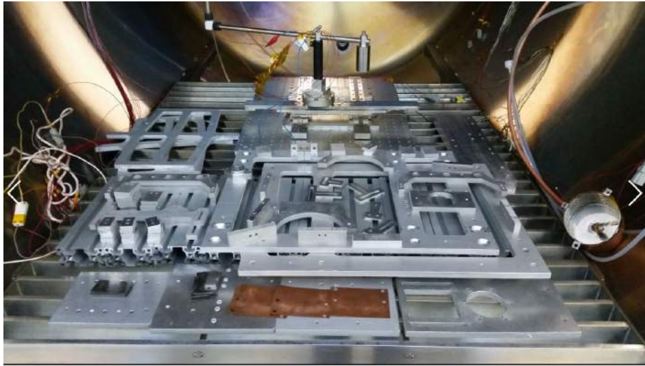
Figure 2.40. Thrust stand components in vacuum chamber
