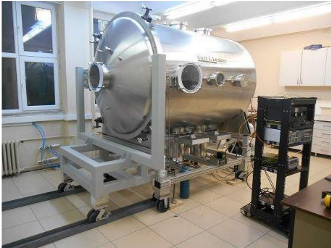
Figure 4.1. BUSTLab vacuum chamber
