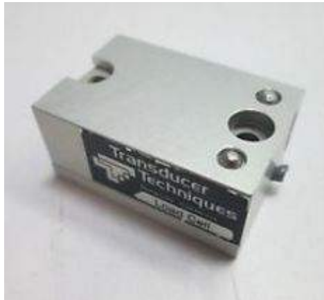
Figure 2.29. Load cell that is used in calibration
