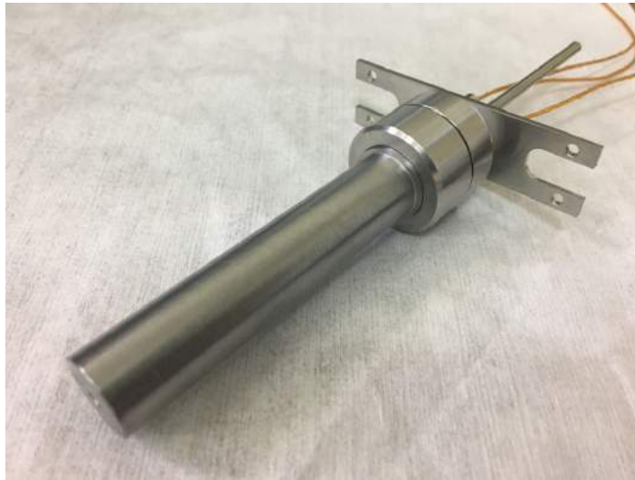
Figure 3.3. BUSTLab hollow cathode
