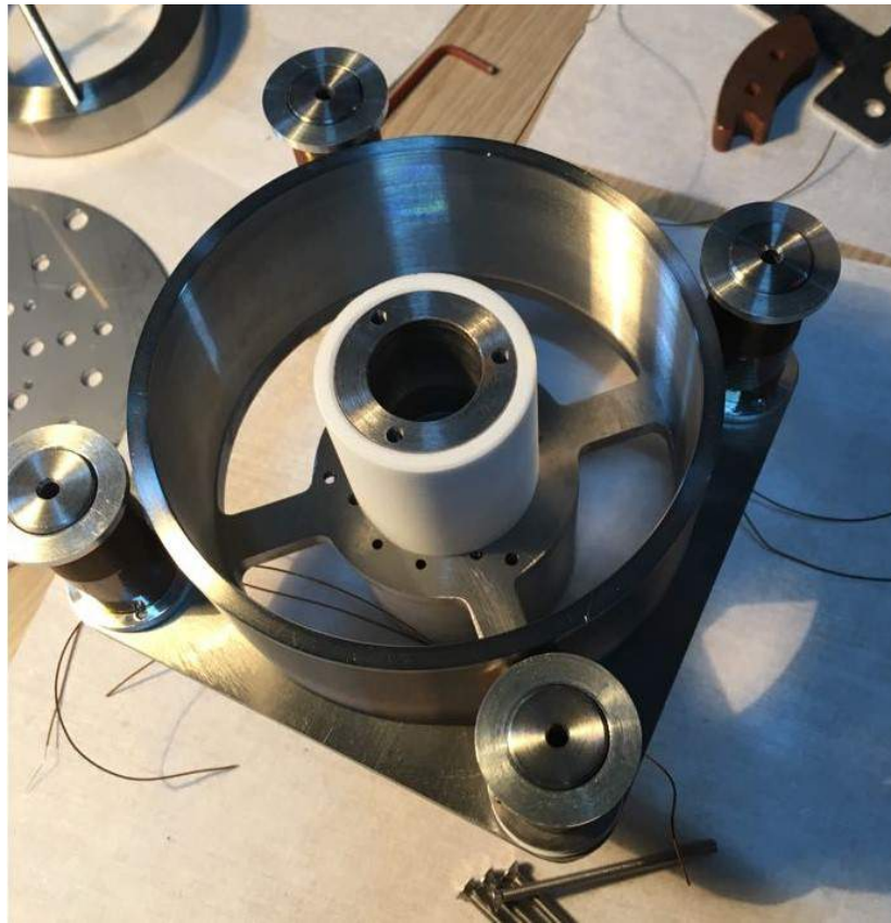
Figure 3.25. Magnetic circuit assembly with inner ceramic spool
