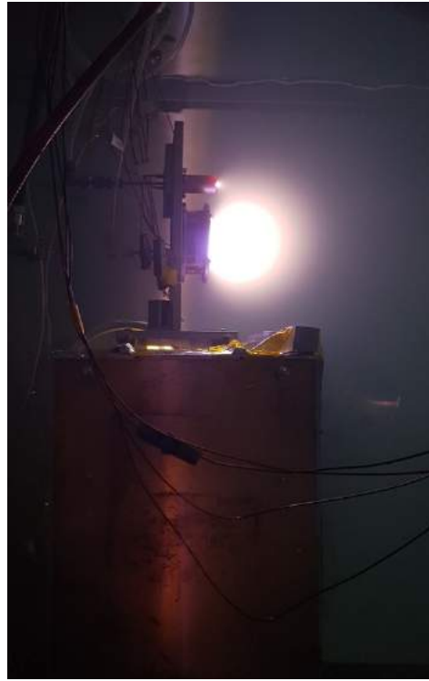
Figure 4.3. HK40 Hall thruster mounted on thrust stand
