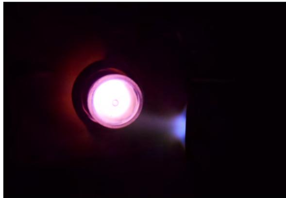
Figure 4.8. Cusped field Hall thruster operating with the RF plasma cathode.
