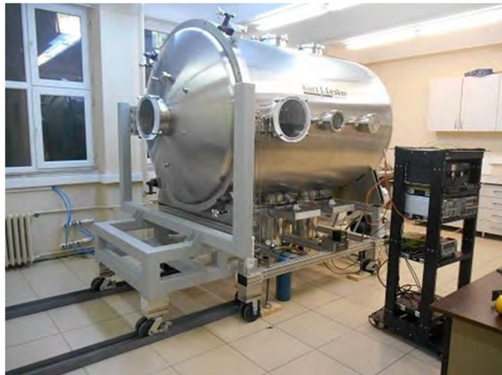
Figure 3.3. BUSTLab vacuum chamber facility.
