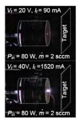
Figure 1.8. Transition mode for 80 W RF power and 2 sccm mass flow rate condition [12].
