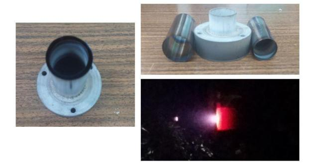
Figure 3.9. Tantalum shields after alumina deposition on their surfaces, and glow of the keeper tube when tantalum shields do not work as planned.
