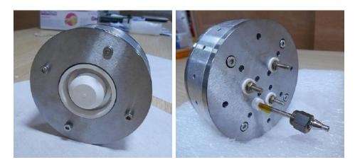
Figure 2.7. HK40 Hall effect thruster (views from the front and the back sides).
