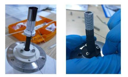
Figure 3.14. The first and the latest heater designs.
