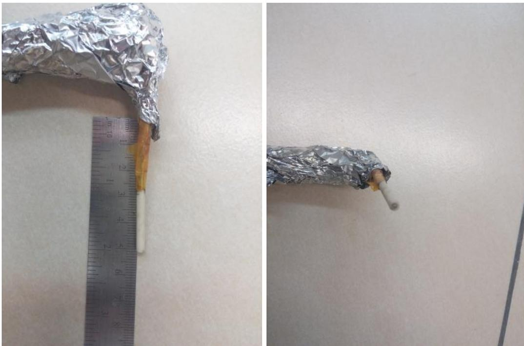
Figure 4.17. Single Langmuir probe constructed for the tests.
