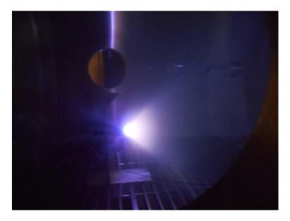
Figure 1.9. CFHT-40 while operating inside the vacuum chamber.
