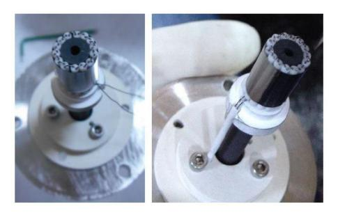
Figure 3.10. The heater wire turning in 14 alumina tubes.
