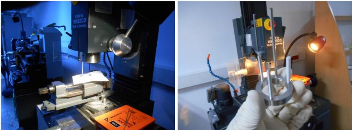
Figure 2.12. Cold mounting for the gas line.
