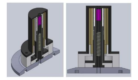
Figure 3.6. The schematic of BUSTLab hollow cathode.
