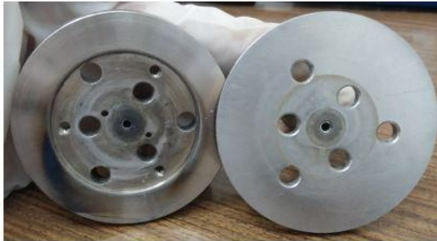
Figure 3.12. The wear on the cathode base.
