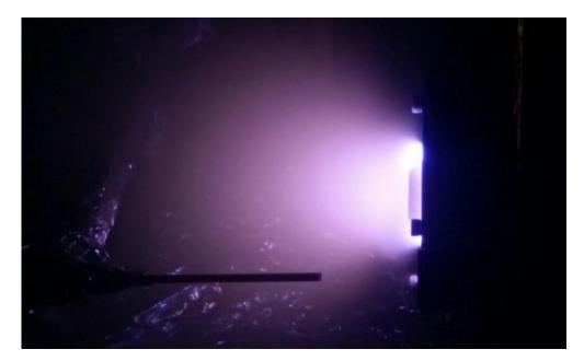
Figure 4.34. HK40 Hall effect thruster with BUSTlab LaB<sub>6</sub> hollow cathode.
