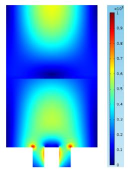
Figure 4: Electric field [V/m] distribution with quartz plate for  $h_s = 75.58$  mm
