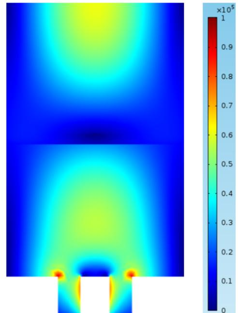
Figure 4: Electric field [V/m] distribution with quartz plate for  $h_s = 75.58$  mm
