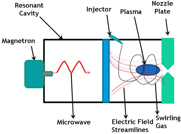
Figure 1: Microwave Electrothermal Thruster System
