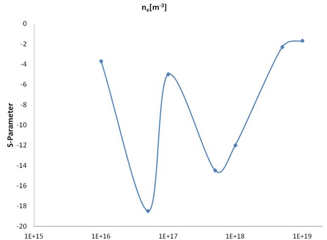
Figure 10: Minimum S-parameter values for different number densities
