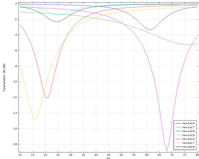
Figure 8: S-parameter vs.  $h_s$  for different number densities
