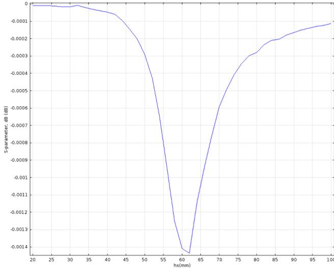
Figure 5: S-parameter vs.  $h_s$  for cavity with separation plate
