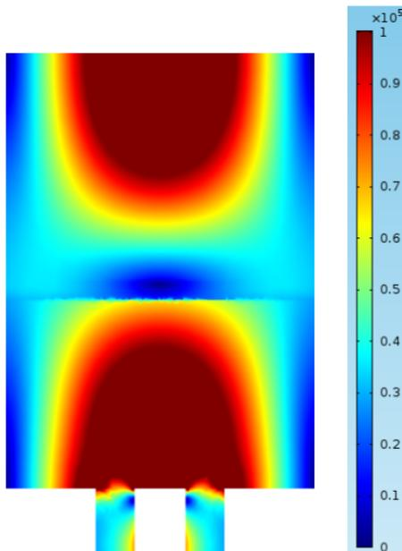
Figure 6: Electric field [V/m] distribution for the cavity with quartz plate for  $h_s= 62$  mm
