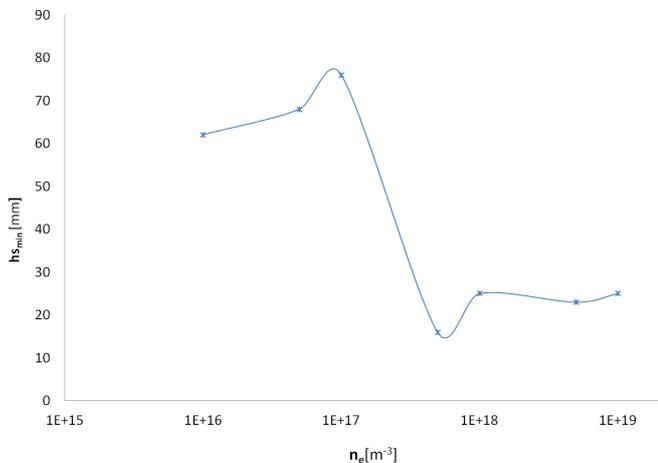
Figure 9: Minimum  $h_s$  values for different number densities
