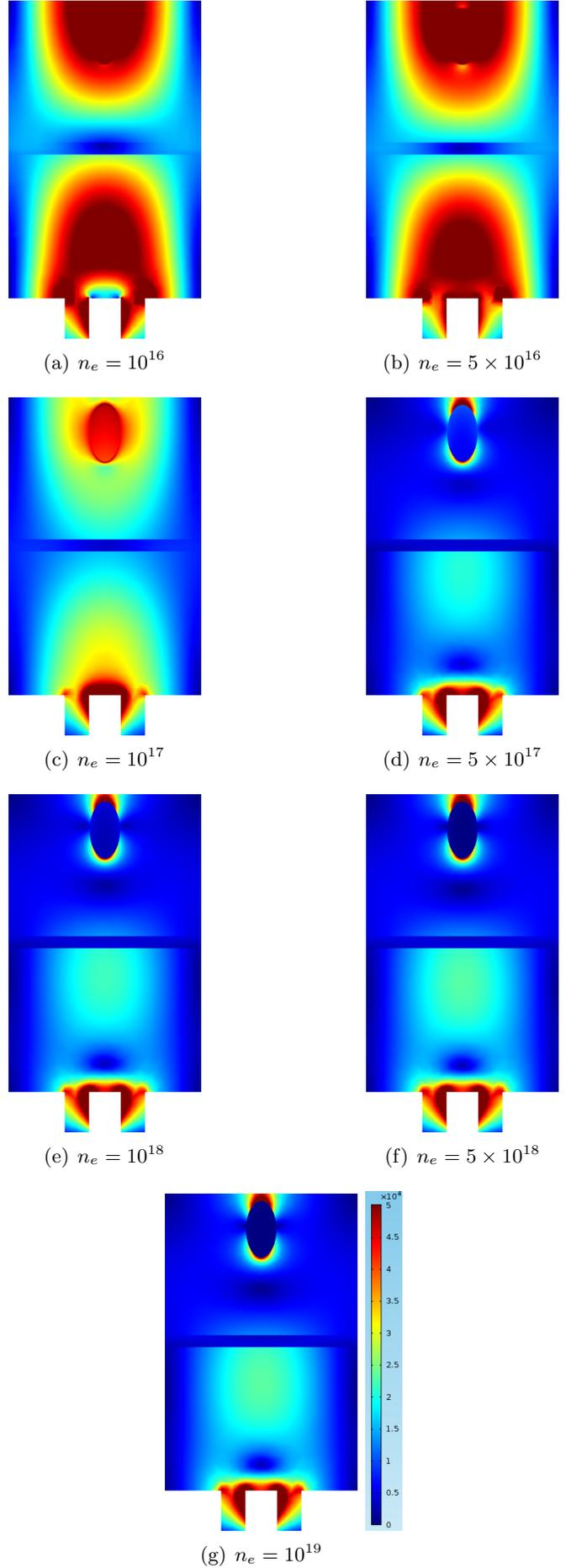
Figure 7: Electric field [V/m] distribution for cavity with plasma disturbance at 2.45 GHz for various  $n_e$  level
