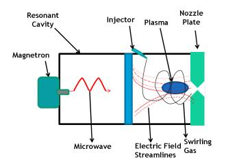
Figure 1: Microwave Electrothermal Thruster System
