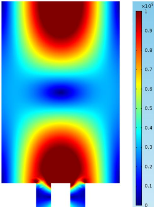
Figure 3: Electric field [V/m] distribution in empty cavity at 2.45 [GHz]
