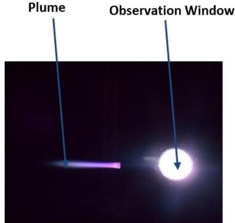
Figure 5. Plasma plume of MET operating inside the BUSTLab vacuum chamber
