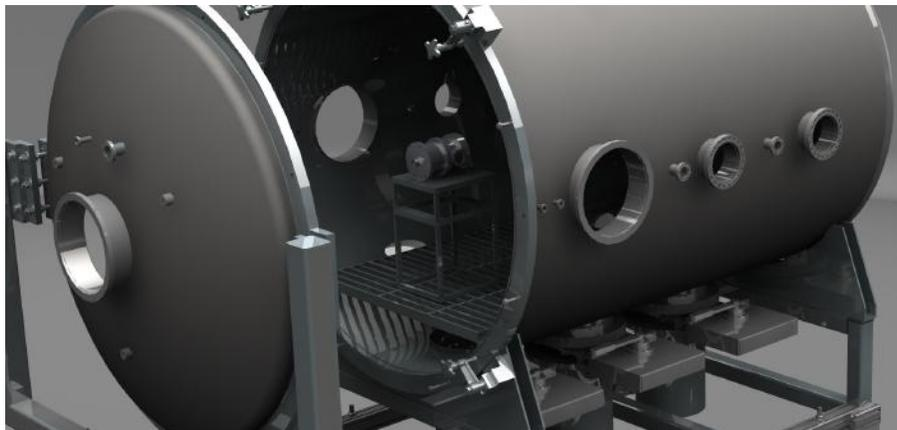
Figure 7. 3D rendering of the MET system on the thrust stand inside the vacuum chamber
