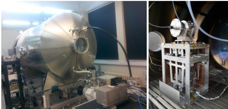
**Figure 4. a) BUSTLab vacuum chamber b) MET on thrust stand before tests,**
