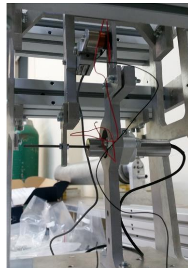
Fig. 10. Sensor assembly: LVDT is in the middle, voice coil and load cell is in the upper part
