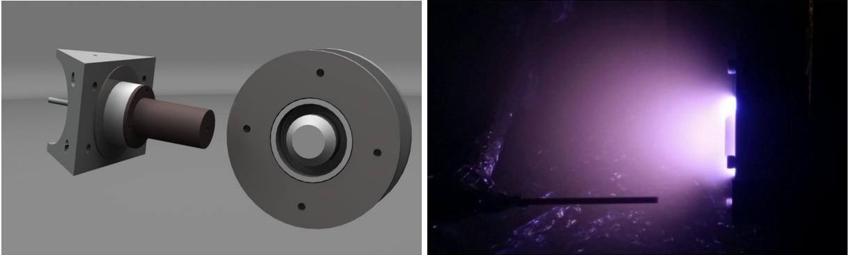
Figure 2: HK40 Hall effect thruster with BUSTlab  $LaB_6$  hollow cathode
