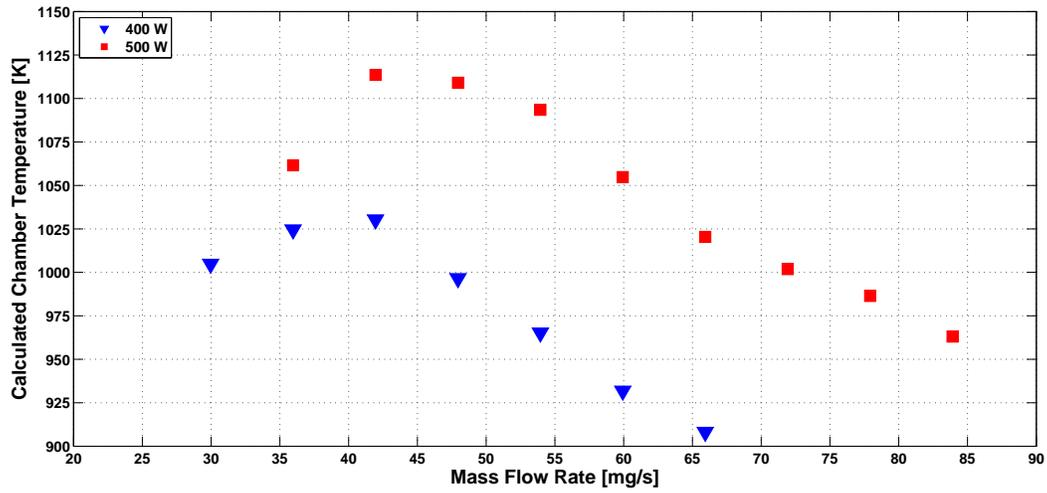
Figure 5. Chamber temperature values at 400 W and 500 W microwave power levels calculated using chamber pressure data.
