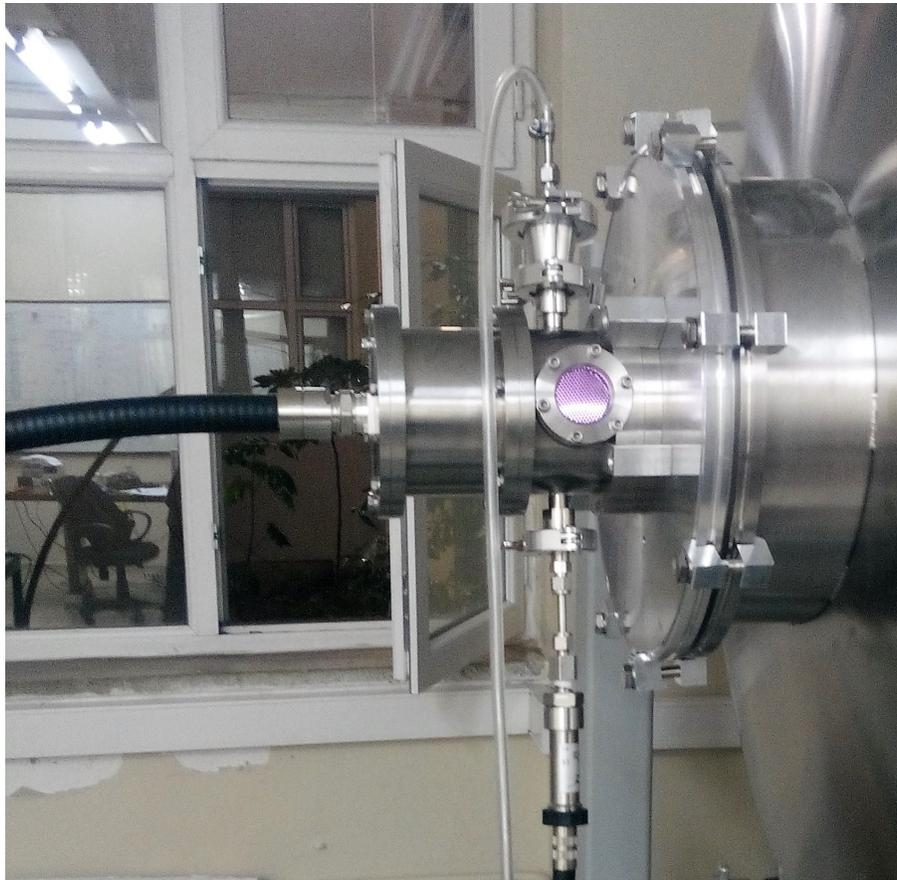
**Figure 2.** BUSTLab MET thruster attached to one of the ports of the BUSTLab vacuum chamber
