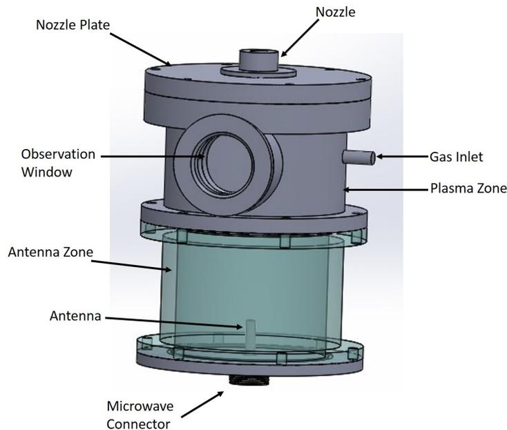
Figure 1. MET Schematic
