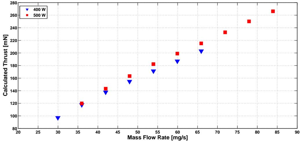
Figure 7. Calculated thrust values at 400 W and 500 W microwave power levels.
