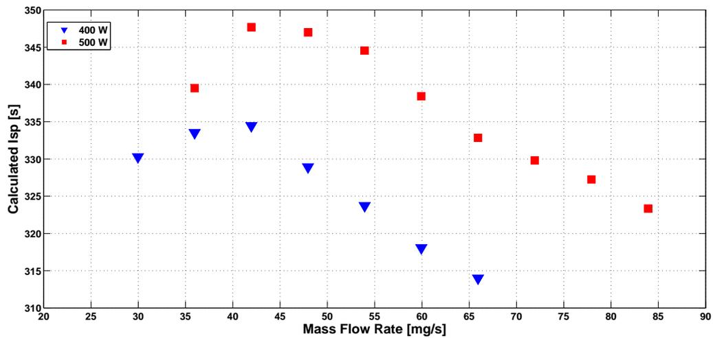
Figure 6. Calculated  $I_{sp}$  values at 400 W and 500 W microwave power levels.
