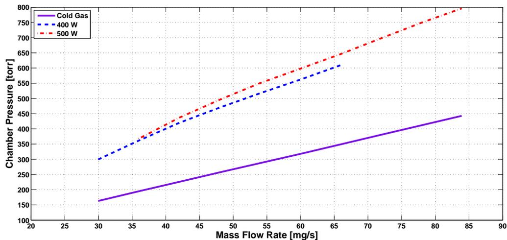
Figure 4. Chamber pressure experimental data for cold gas, 400 W and 500 W microwave power levels.
