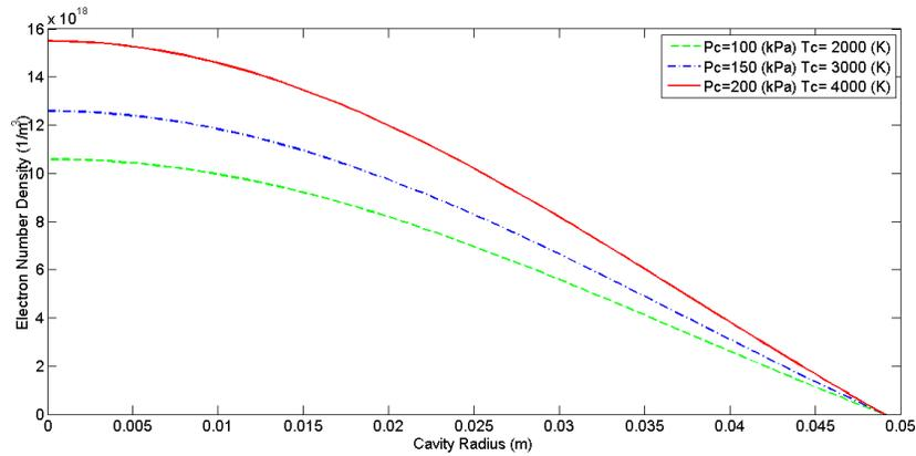
**Figure 7. Electron Density Radial Distribution**
