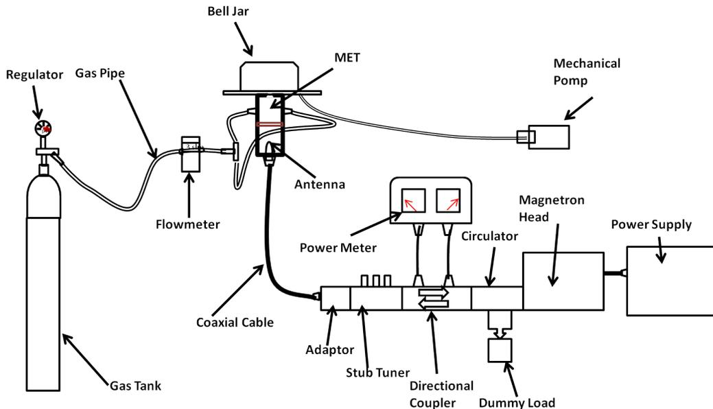
Figure 2. Experimental Setup
