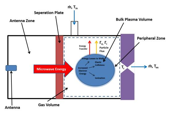
Figure 6. Schematic of the mass and energy transport for the plasma in the resonant cavity of MET
