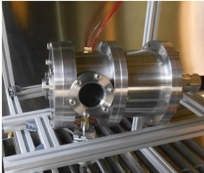
Figure 1. BUSTLab microwave-electrothermal-thruster on a stand inside the BUSTLab vacuum chamber
