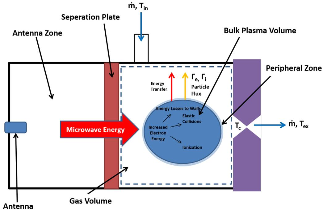
Figure 6. Schematic of the mass and energy transport for the plasma in the resonant cavity of MET
