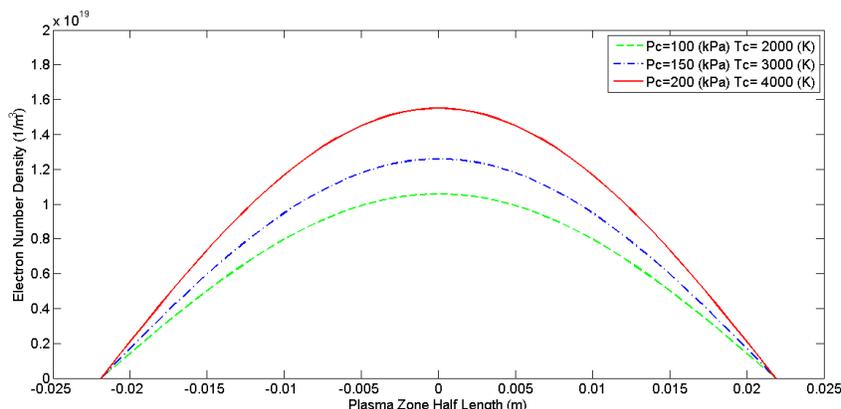
Figure 8. Electron Number Density Axial Distribution
