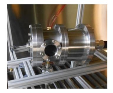
Figure 1. BUSTLab microwave-electrothermal-thruster on a stand inside the BUSTLab vacuum chamber
