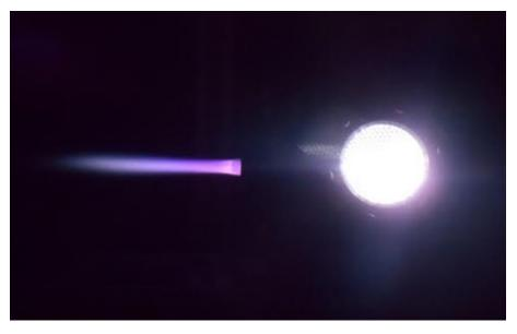
Figure 5. Plasma plume of MET operating inside the BUSTLab vacuum chamber
