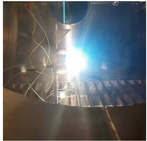
Fig. 10. The first testing of the HK40 Hall effect thruster inside the BUSTLab vacuum chamber
