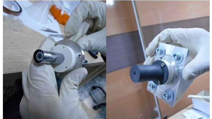
Fig. 7. LaB 6 hollow cathode during and after assembly
