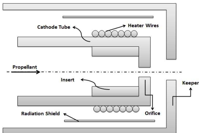
Figure 1: Schematic of hollow cathode
