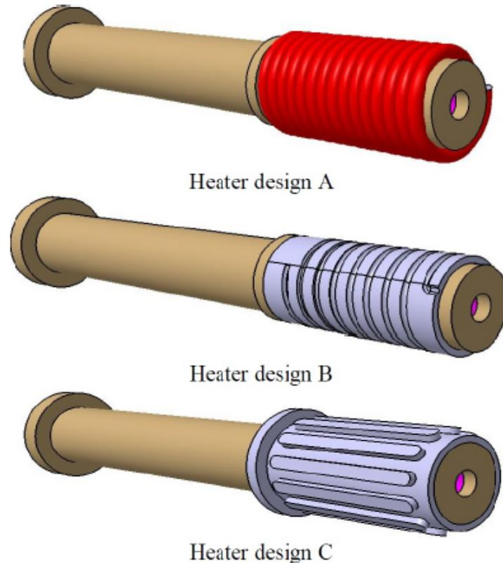
Figure 4: Solid models of different heater designs
