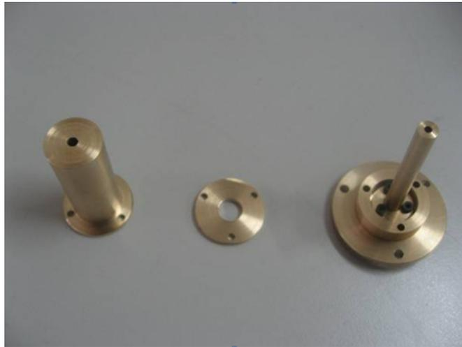
Figure 6: Prototype hollow cathode made of brass
