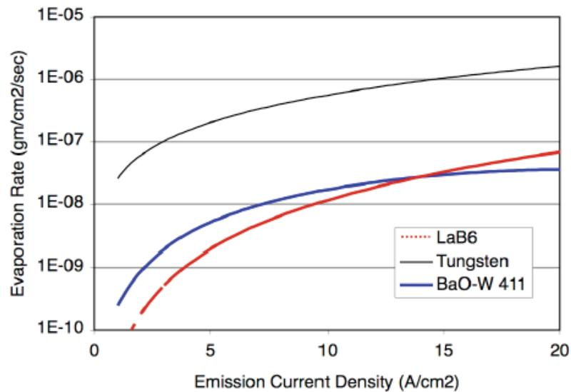
Figure 2: Evaporation of different emissive materials [Goebel and Chu, 2011]
